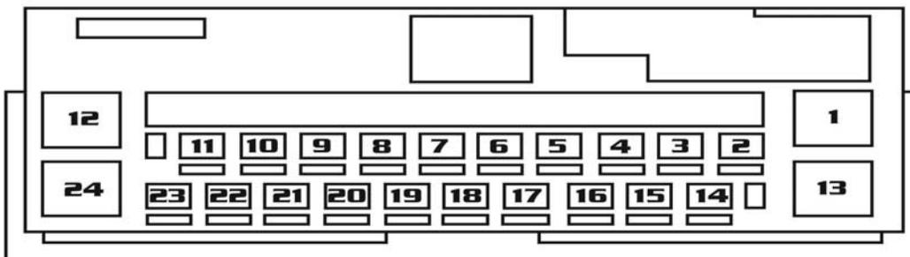
This is the pin view of the connector in the vehicle
